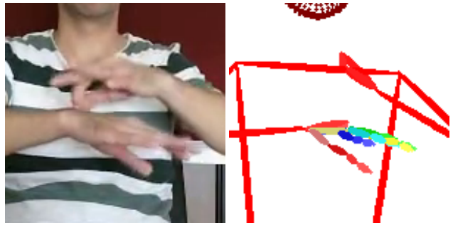
Figure 3. Example of hands interaction, where the pose estimation fails for one of the hands (Holistic).
